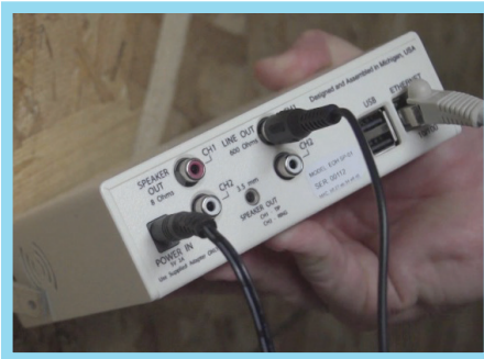
Output to phone system: Line Out CH 1 RCA.
